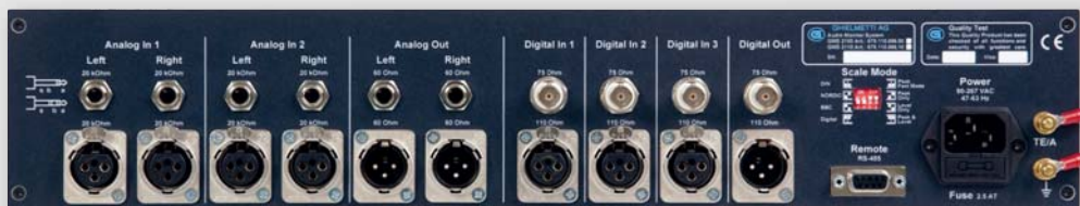
On analog connections you'll find XLR and servo symmetrical jack plugs. Digital signals are switched in and out of the unit by XLR (AES/EBU) or by BNC plugs in S/PDIF-format. The 4 DIP switches allow the scaling of the level meter and a RS-485 interface is provided for a remote control of the unit.
